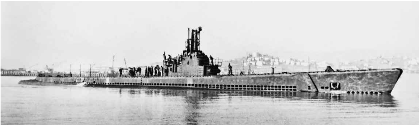
USS Trigger (SS 237) in carrier-hunting mid-war fighting form. This is essentially how she appeared at the time of the events described here—fairwater cut down to reduce silhouette, guns added to the cigarette deck and forward of the bridge. In all respects, ready for action.
